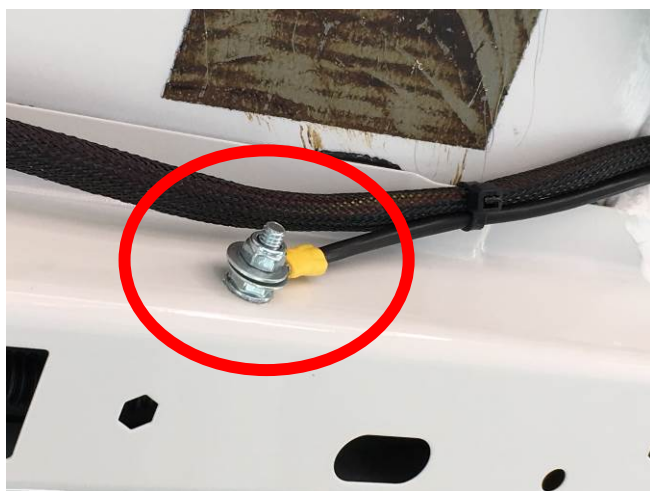
Figure 13: Earth connection to body (AC 3000)
